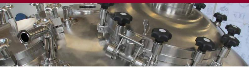
Vertical pressure vessel in cylindrical form with conical bottom and torispherical end. The pressure vessel is manufactured according to the PED (97/23/EC), PED Class III, Module H, ATEX Zone 2 outside.
